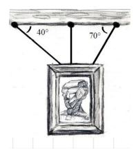
1. Find the mass m of the painting. The tension in the leftmost rope is 7.2 N, in the middle rope it is 16 N, and in the rightmost rope it is 16 N.
